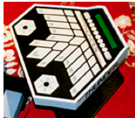
FIG. 3 – The Thunder controller by Don Buchla. Each strip is sensitive to both finger location and pressure in a continuous manner. It provides for polyphonic control of continuous variables
